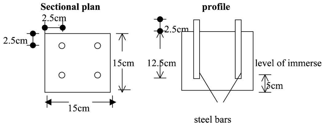
Fig. 1. Schematic representation of reinforced concrete specimens for corrosion tests.
