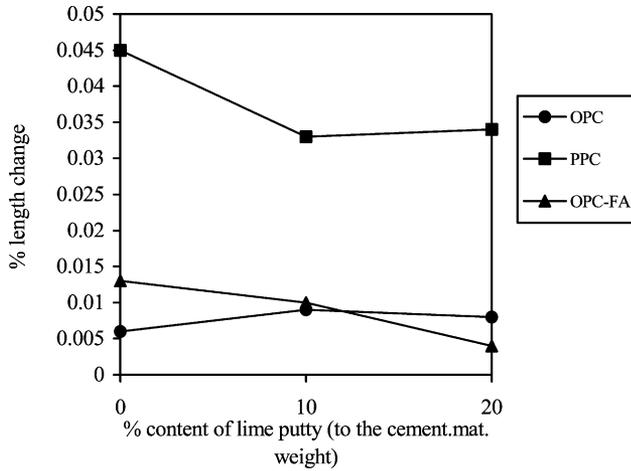
Fig. 4. Effect of lime putty addition on length change of hardened concrete.
