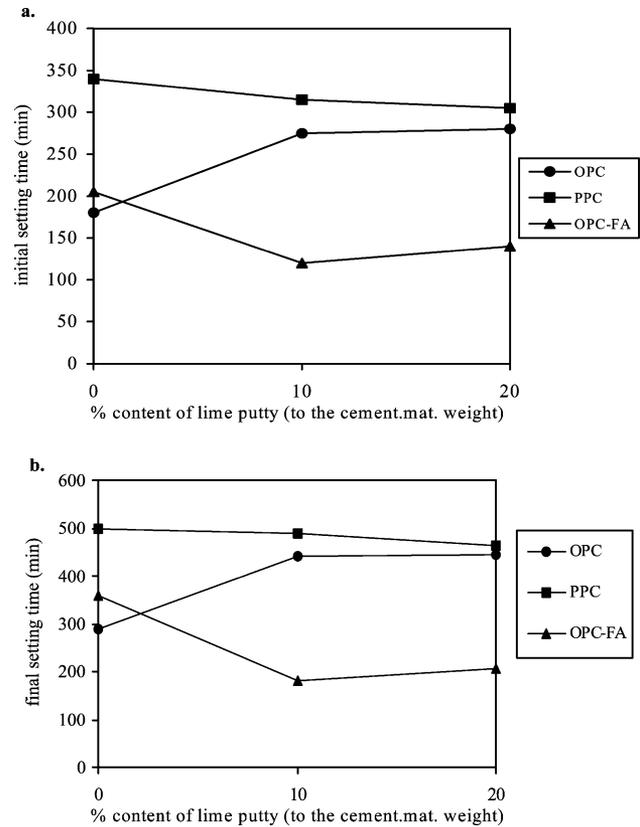
Fig. 3. Effect of lime putty addition on initial (a) and final (b) setting time of concrete.
