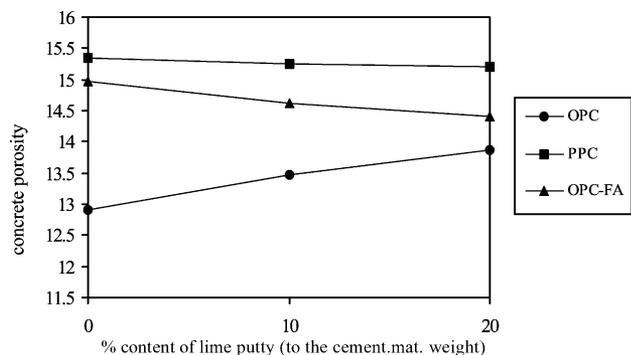
Fig. 5. Effect of lime putty addition on concrete porosity.
