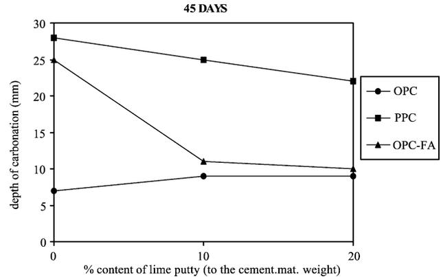
Fig. 6. Effect of lime putty addition on concrete carbonation for different cement types.
