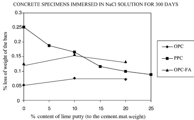
Fig. 8. Effect of lime putty addition on corrosion resistance of reinforcing bars.
