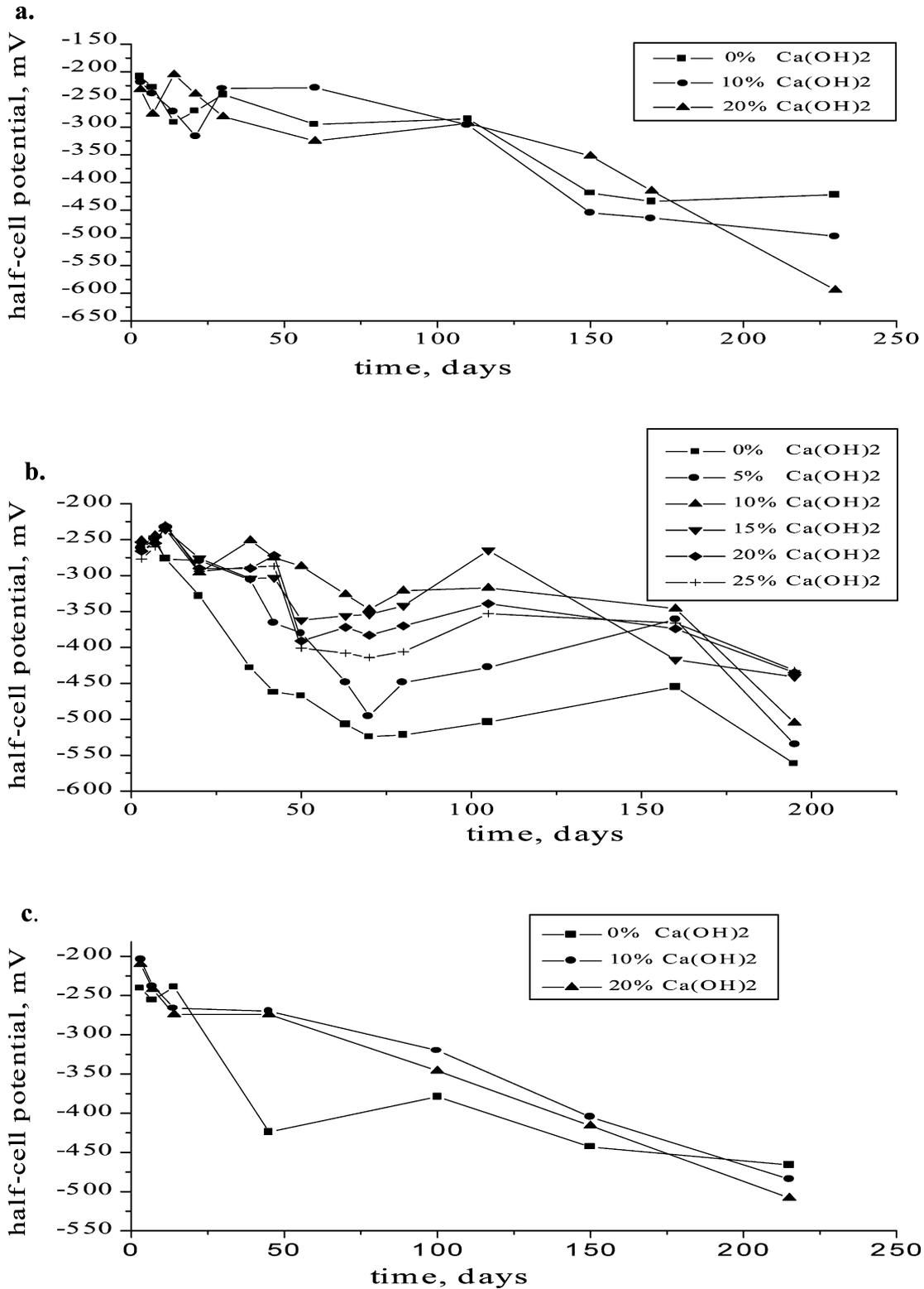
Fig. 7. Half-cell potentials of reinforcing bars of concrete immersed in 3.5% NaCl solution. (a) OPC; (b) PPC; (c) OPC-FA.
