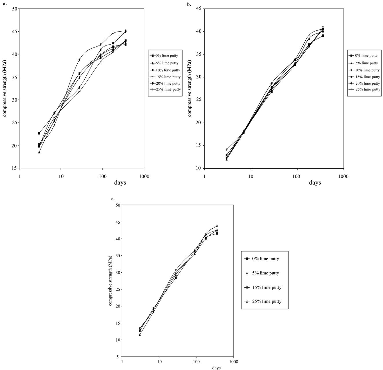
Fig. 2. Effect of lime putty addition on compressive strength of concrete for different cementitious materials. (a) OPC; (b) PPC; (c) OPC-FA.
