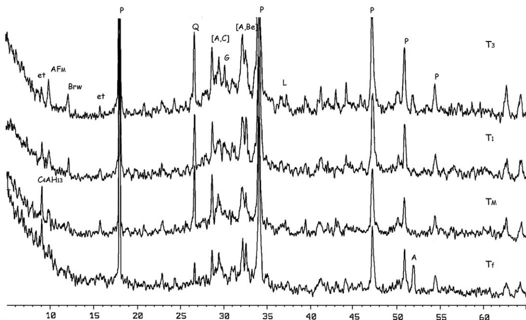
Fig. 4. XRD patterns of hydrated pastes after 7 days of hydration. (The following notations were used for the various minerals identified: et: ettringite,  $AF_m$ : monosulphate, P: portlandite, Br: Brownmillerite, Q: quartz, L: lime, C: calcite, G: gypsum, A:  $C_3S$ , Be:  $C_2S$ ).
