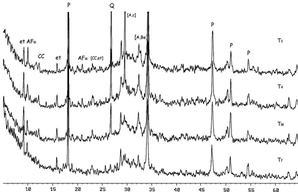
Fig. 5. XRD patterns of hydrated pastes after 90 days of hydration. (The following notations were used for the various minerals identified: et: ettringite, AF<sub>m</sub>: monosulphate, P: portlandite, Q: quartz, Cc: C<sub>4</sub>A C H<sub>11</sub>, C: calcite, G: gypsum, A: C<sub>3</sub>S, Be: C<sub>2</sub>S).
