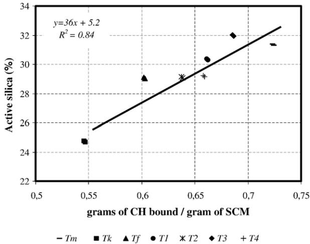
Fig. 1. Chapelle test results for initial and blended ashes in relation to their active silica content.
