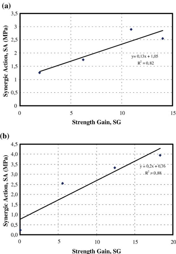
Fig. 3. Strength gain (SG) versus synergic action (SA) values for (a) T<sub>1</sub> and (b) T<sub>3</sub> ternary cements.
