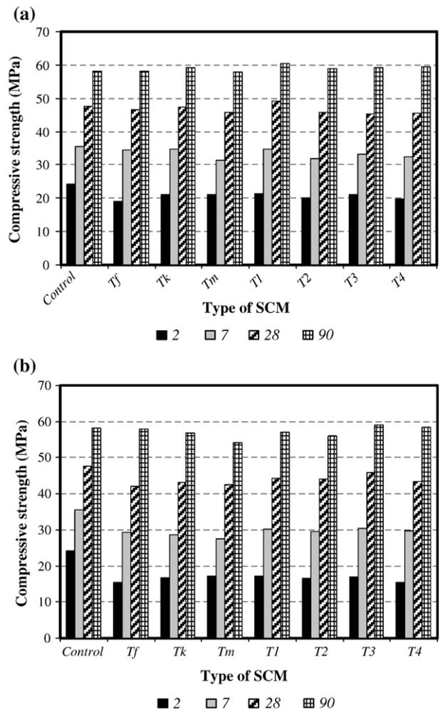
Fig. 2. Compression test results for (a) 20% and (b) 30% by weight cement replacement.
